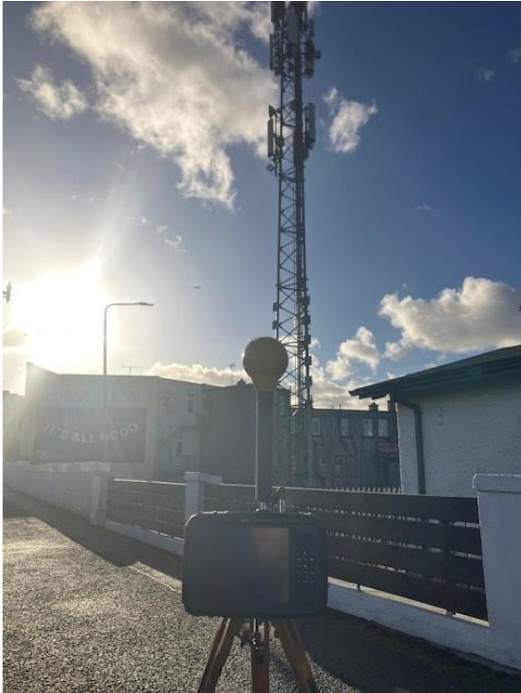
Photo 2. Frequency selective measurement location looking towards antennas
