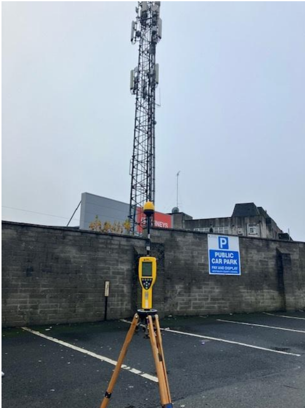
Photo 1. Broadband Measurement location looking towards antennas
