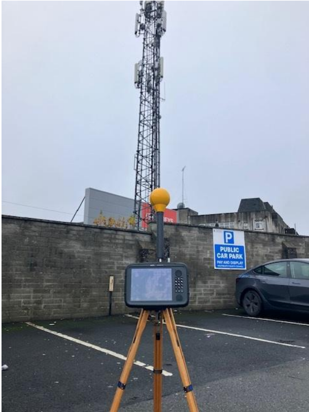
Photo 2. Frequency selective measurement location looking towards antennas
