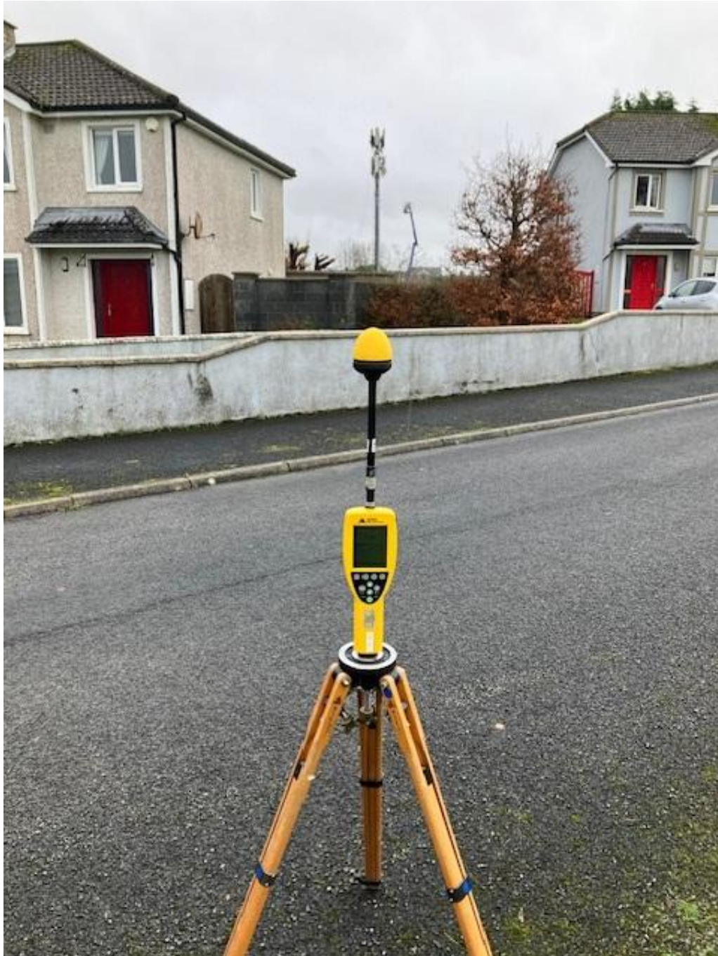
Photo 1. Broadband Measurement location looking towards antennas
