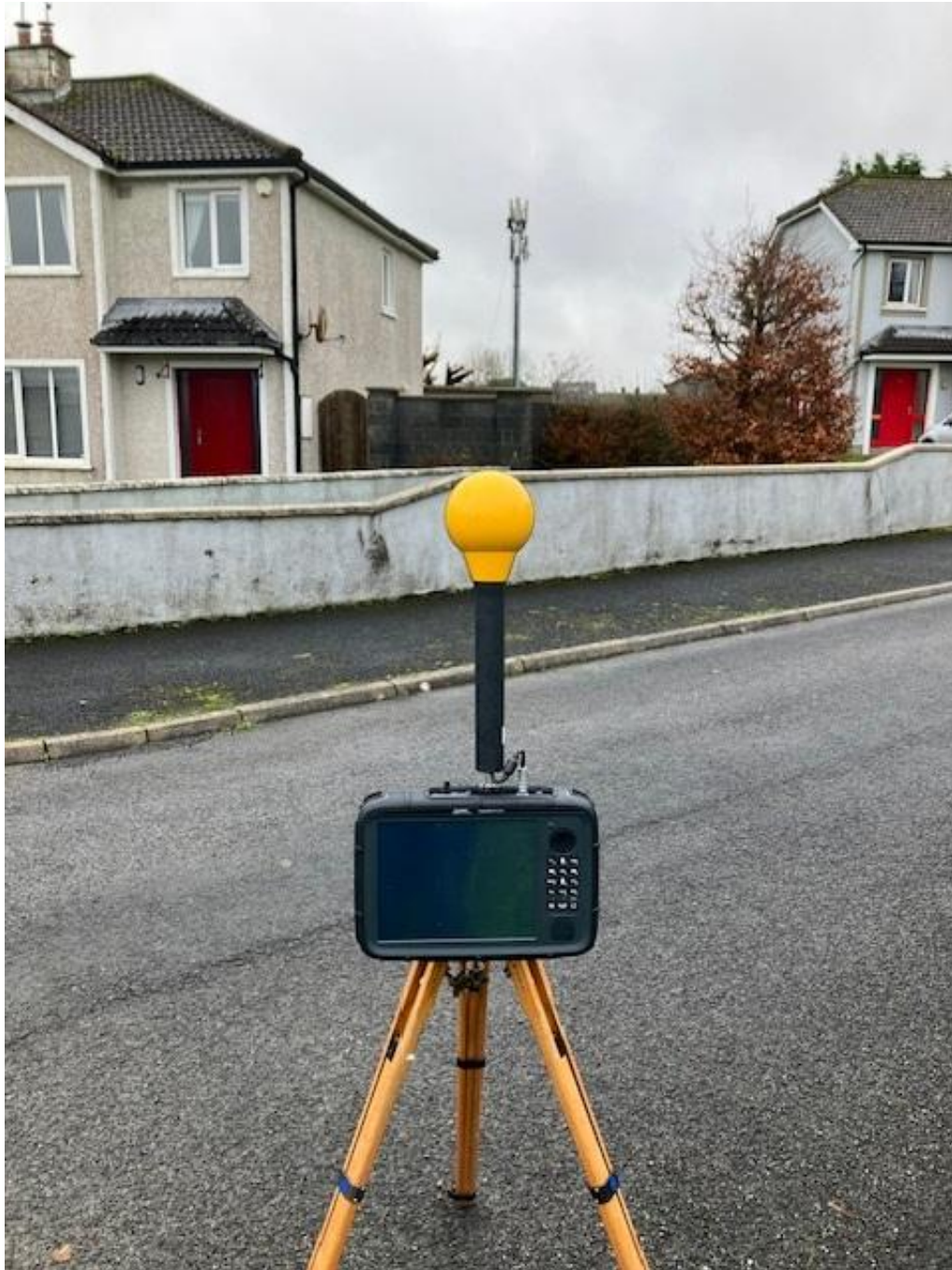
Photo 2. Frequency selective measurement location looking towards antennas
