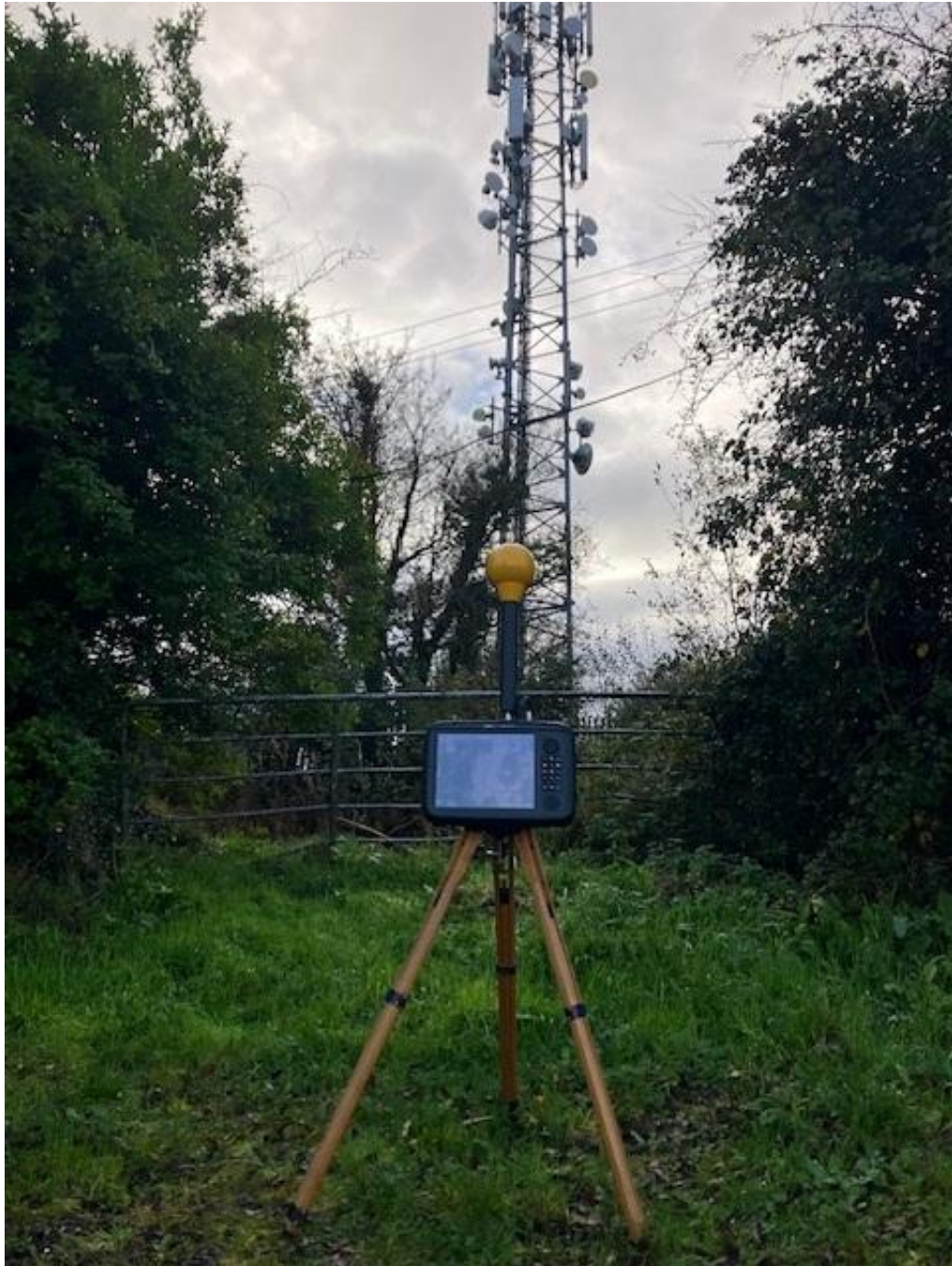
Photo 2. Frequency selective measurement location looking towards antennas
