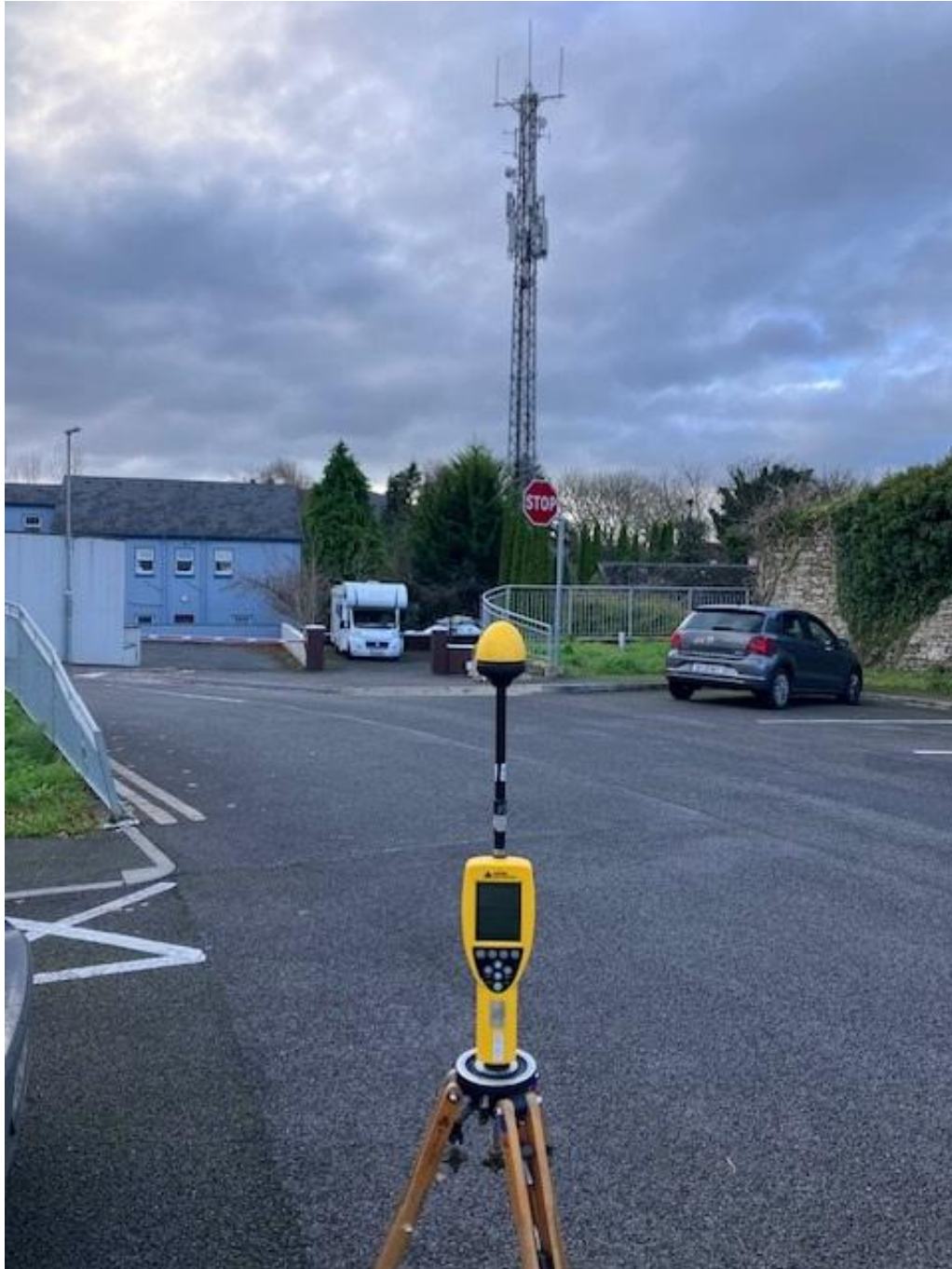
Photo 1. Broadband Measurement location looking towards antennas
