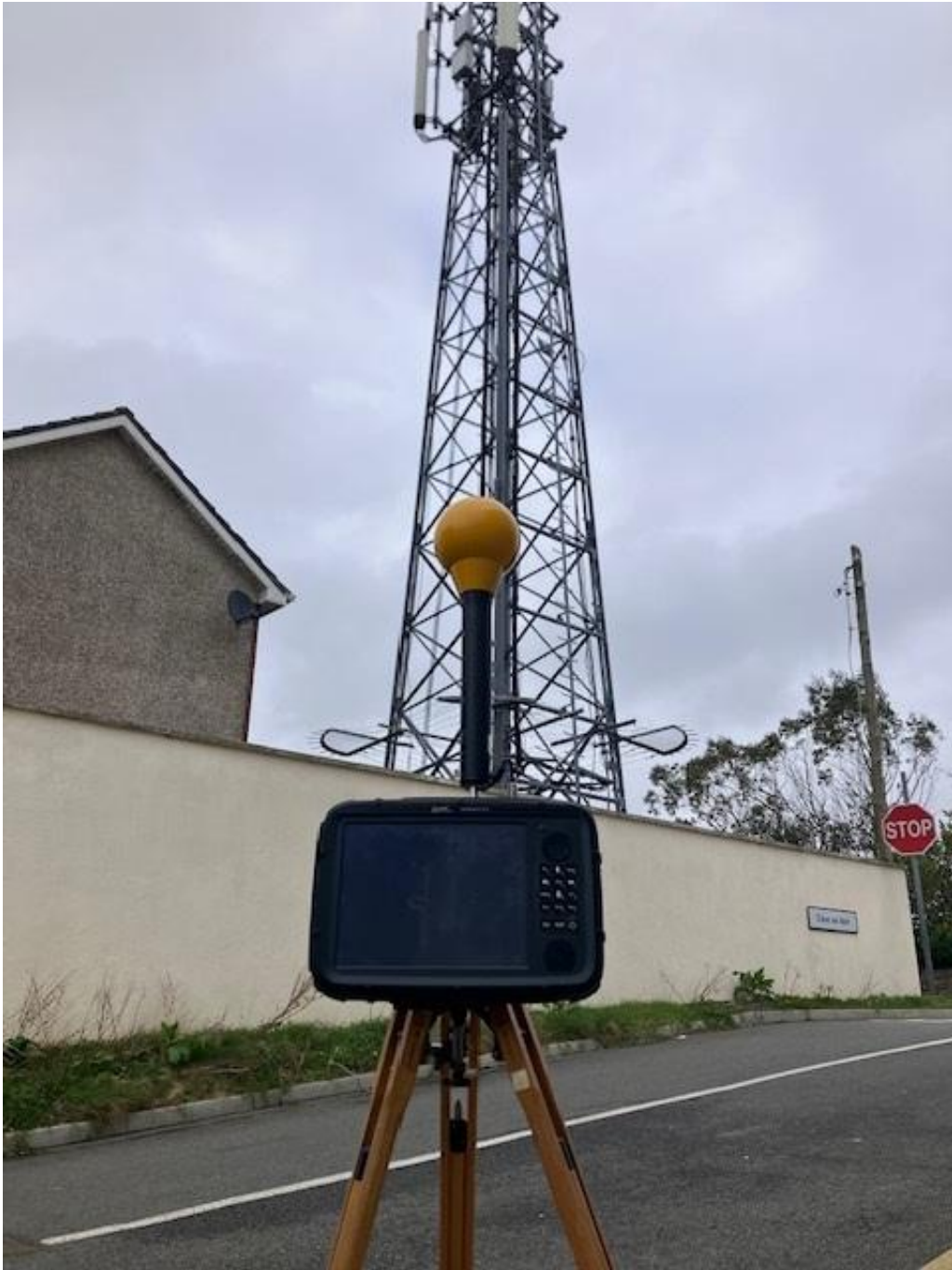
Photo 2. Frequency selective measurement location looking towards antennas
