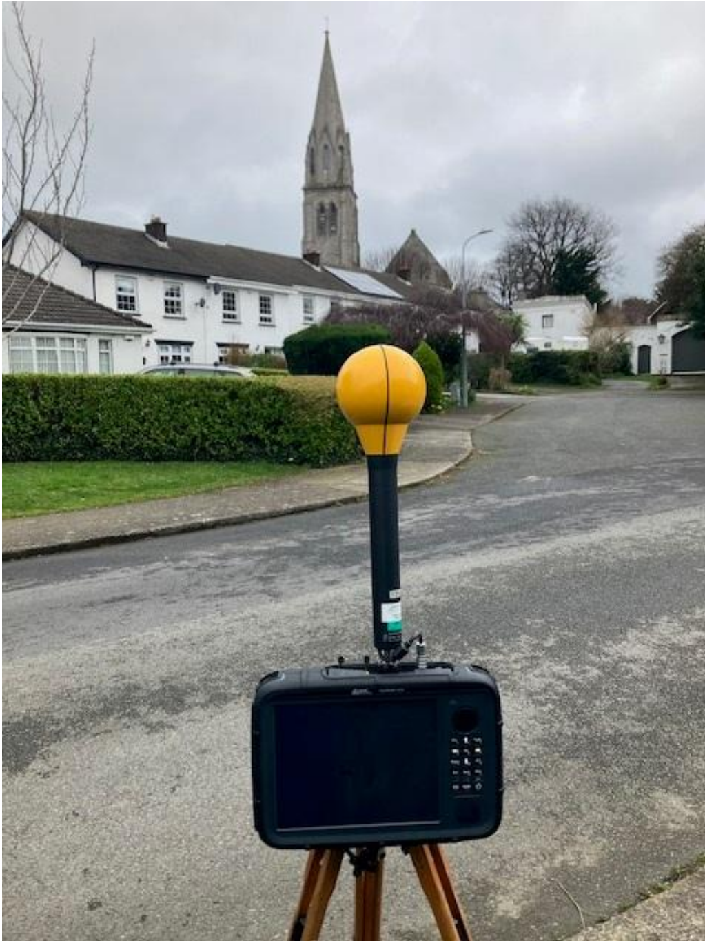
Photo 2. Frequency selective measurement location looking towards antennas
