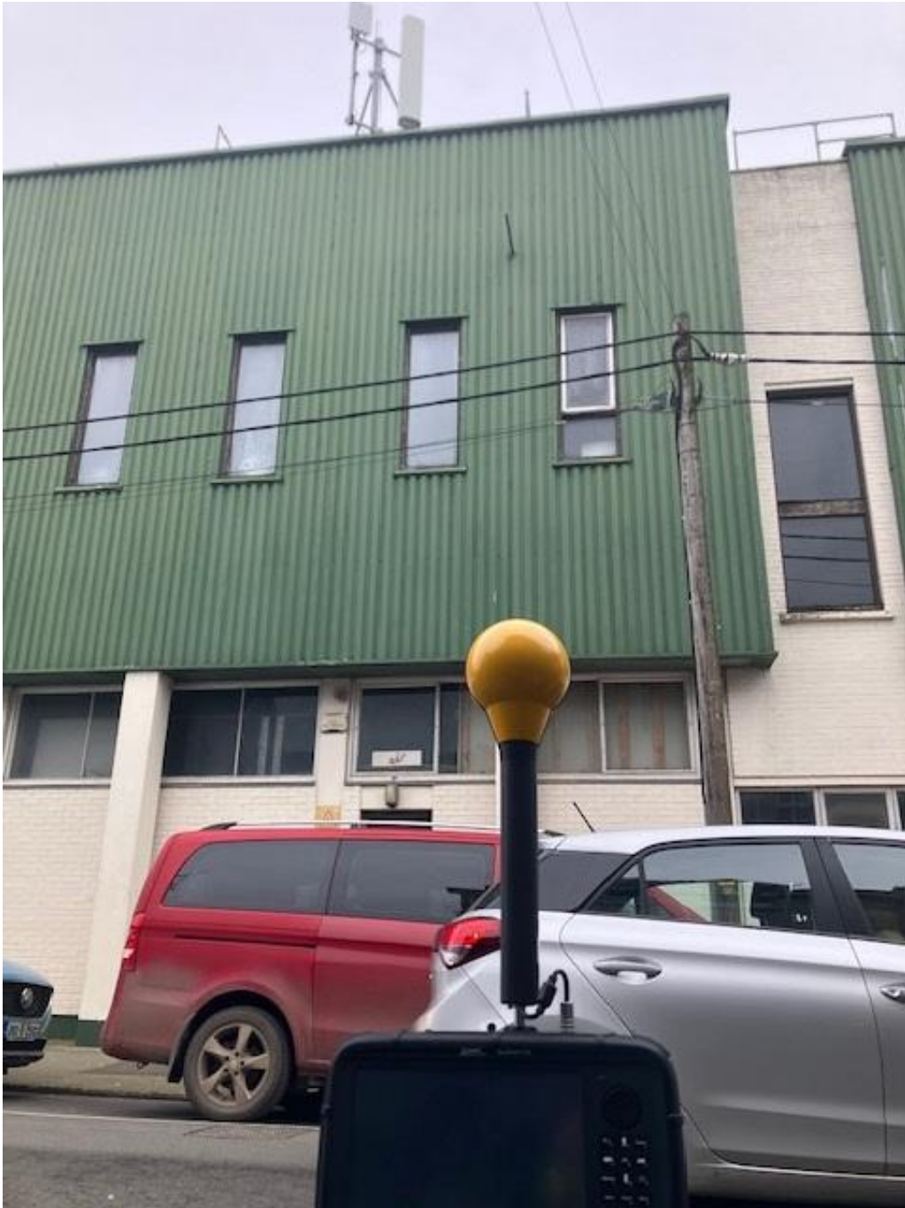
Photo 2. Frequency selective measurement location looking towards antennas
