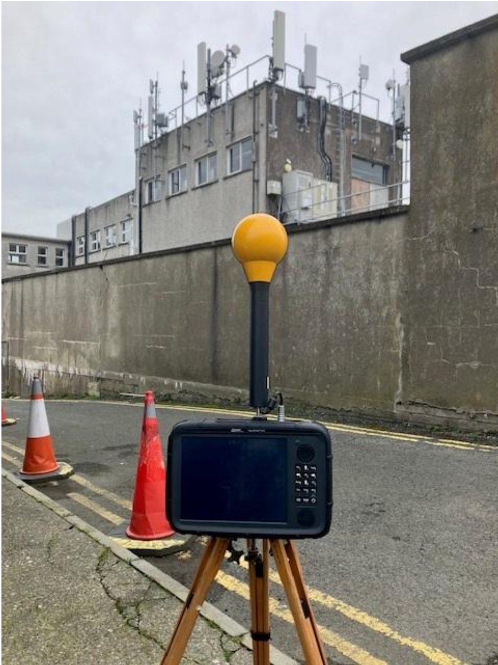
Photo 2. Frequency selective measurement location looking towards antennas
