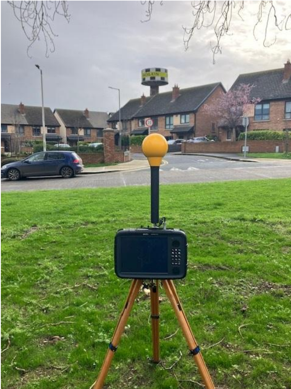
Photo 2. Frequency selective measurement location looking towards antennas
