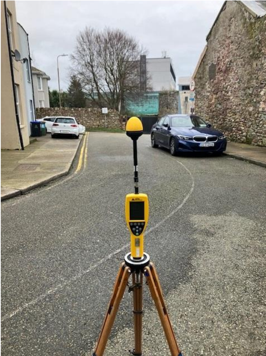
Photo 1. Broadband Measurement location looking towards antennas
