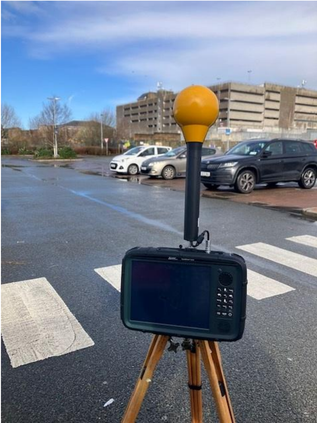
Photo 2. Frequency selective measurement location looking towards antennas
