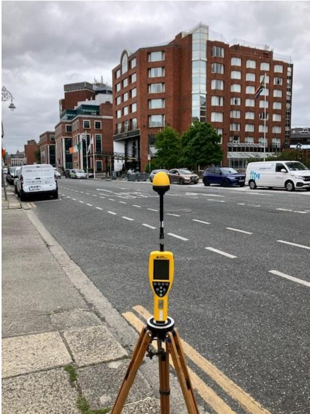
Photo 1. Broadband Measurement location looking towards antennas
