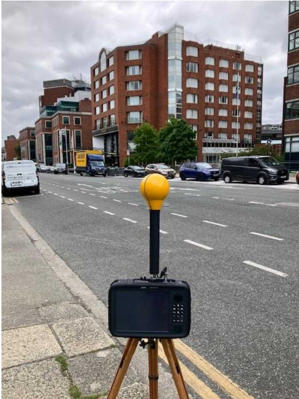
Photo 2. Frequency selective measurement location looking towards antennas
