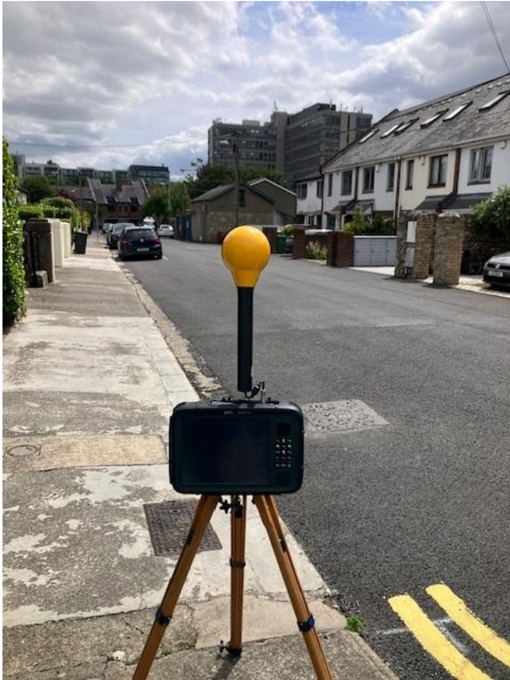
Photo 2. Frequency selective measurement location looking towards antennas
