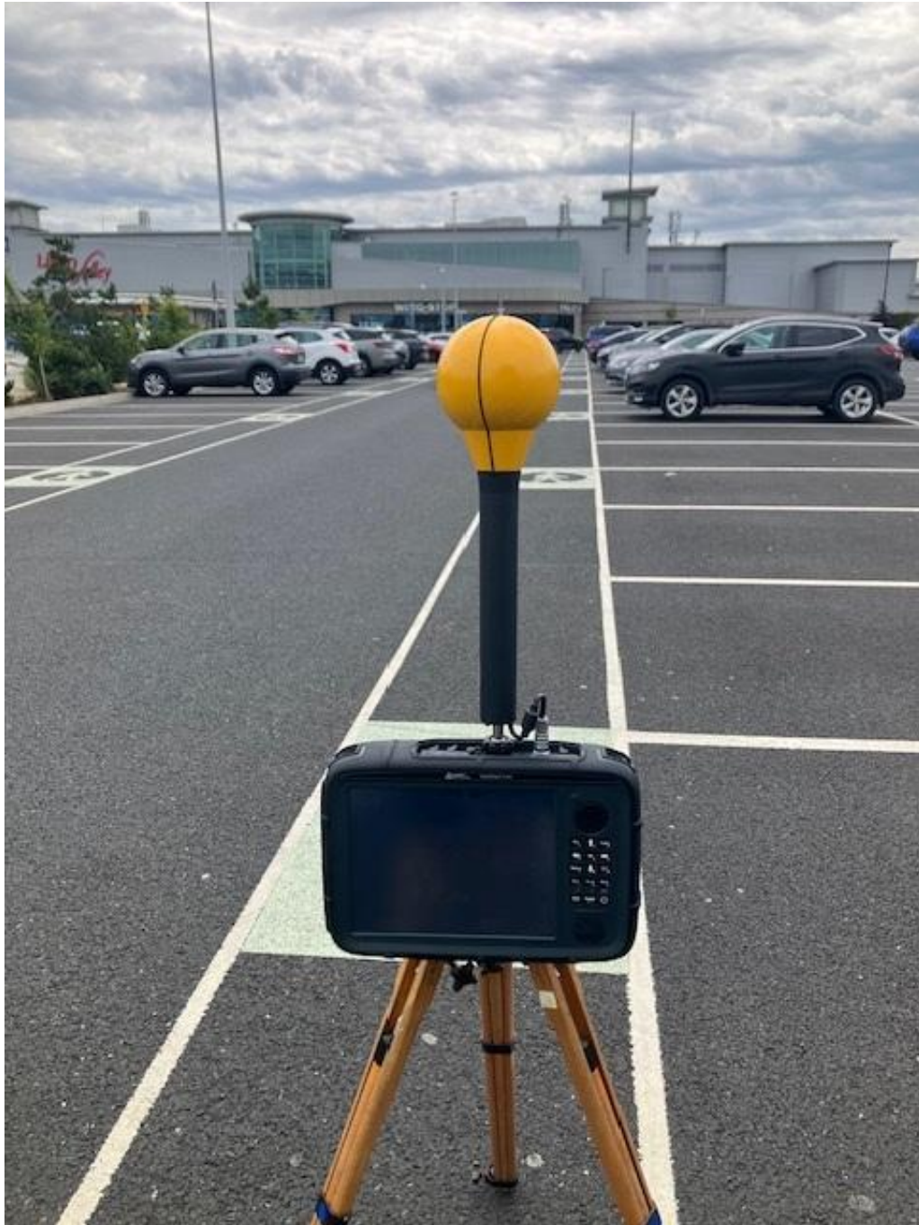
Photo 2. Frequency selective measurement location looking towards antennas
