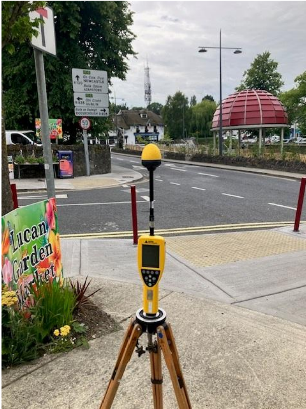
Photo 1. Broadband Measurement location looking towards antennas
