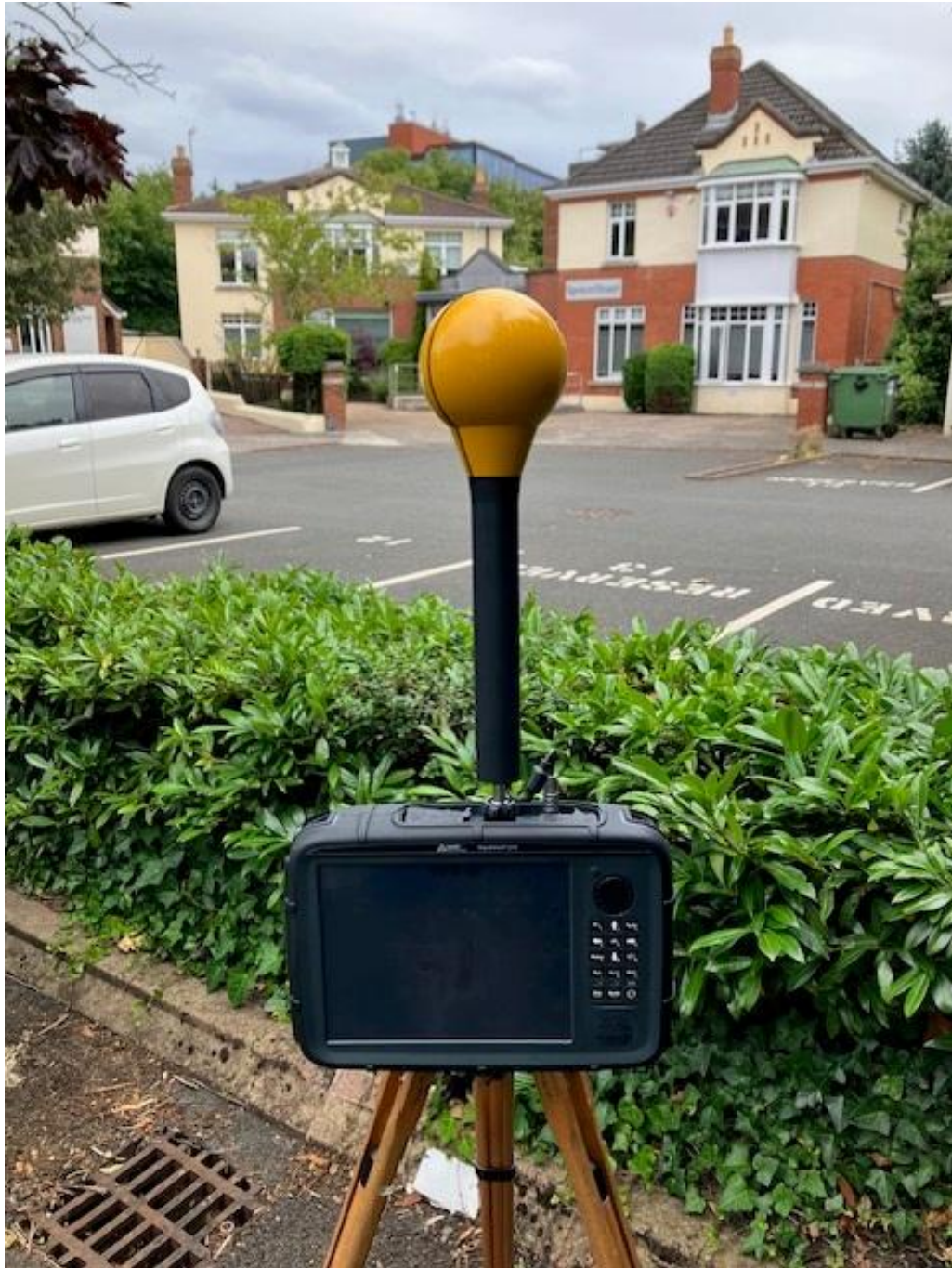
Photo 2. Frequency selective measurement location looking towards antennas
