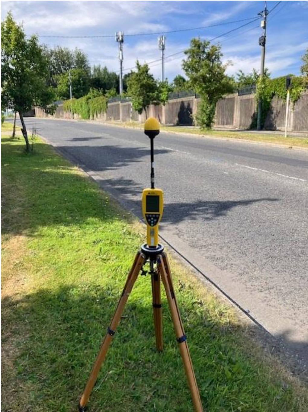
Photo 1. Broadband Measurement location looking towards antennas
