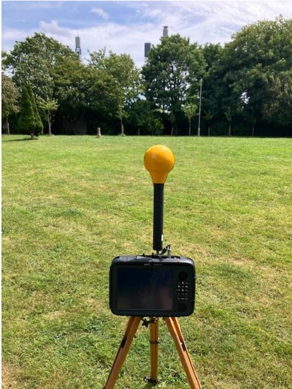
Photo 2. Frequency selective measurement location looking towards antennas
