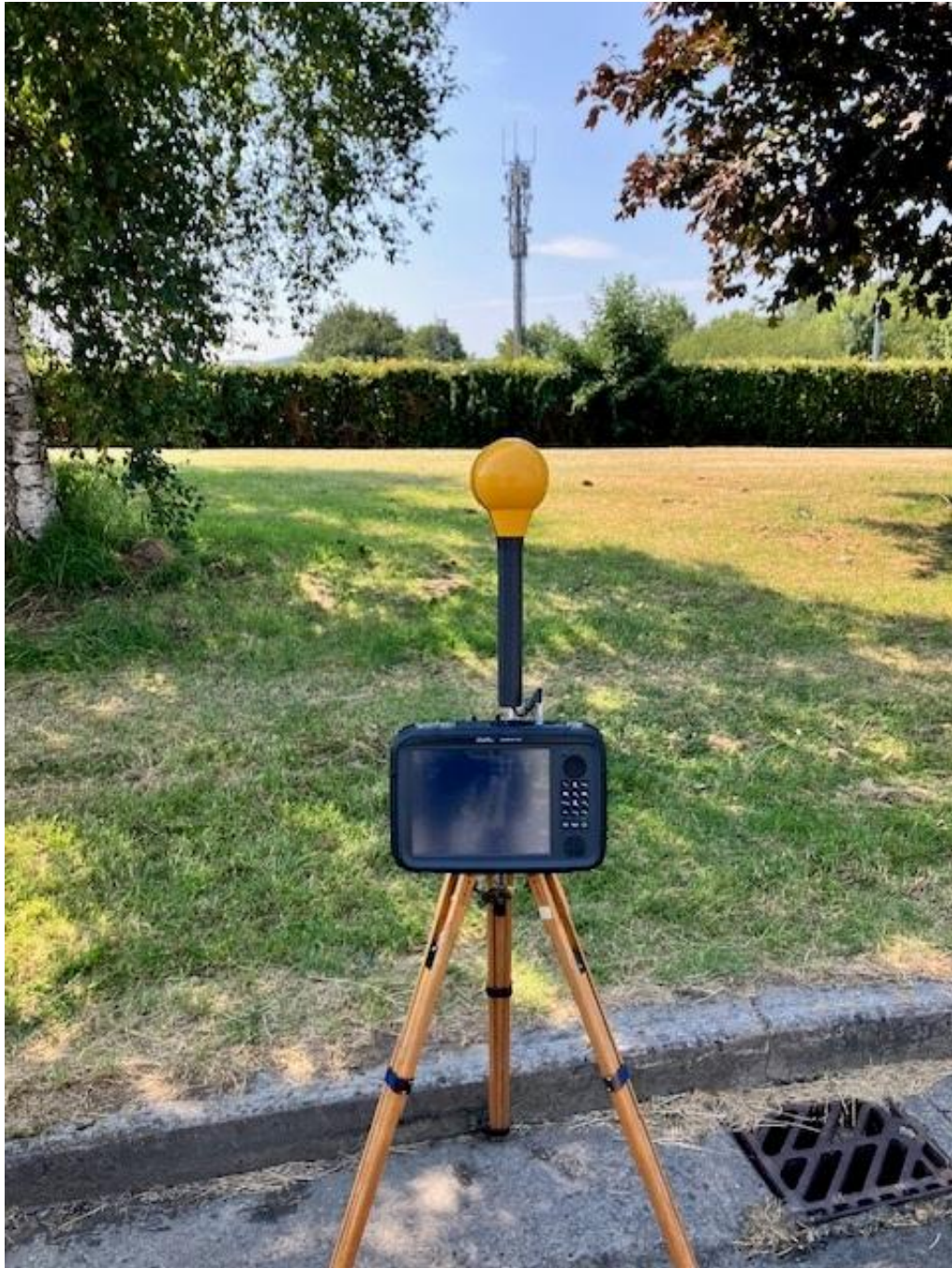
Photo 2. Frequency selective measurement location looking towards antennas
