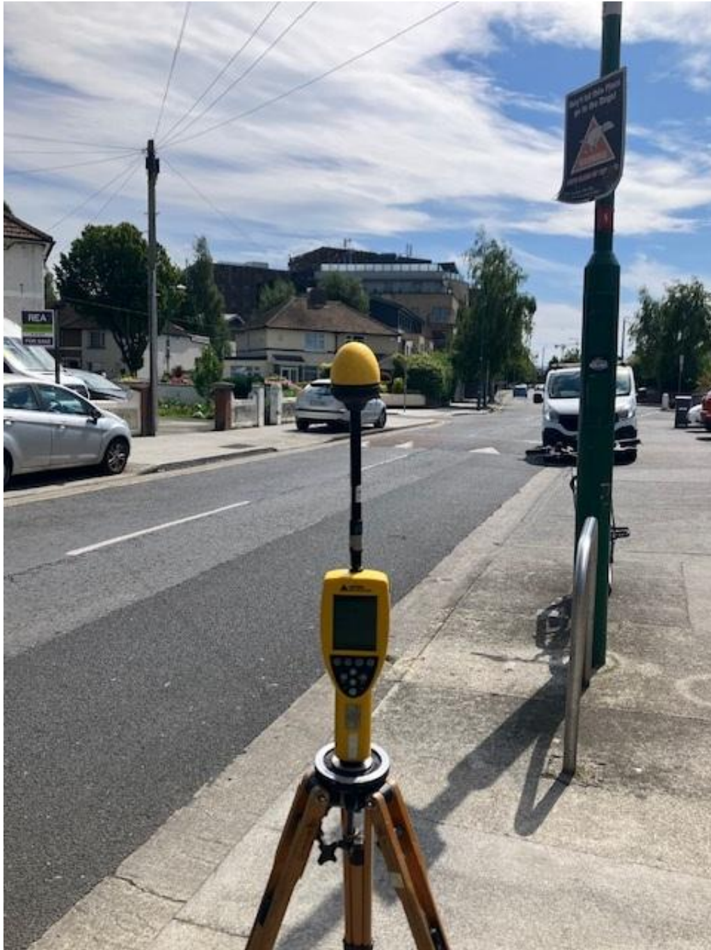
Photo 1. Broadband Measurement location looking towards antennas
