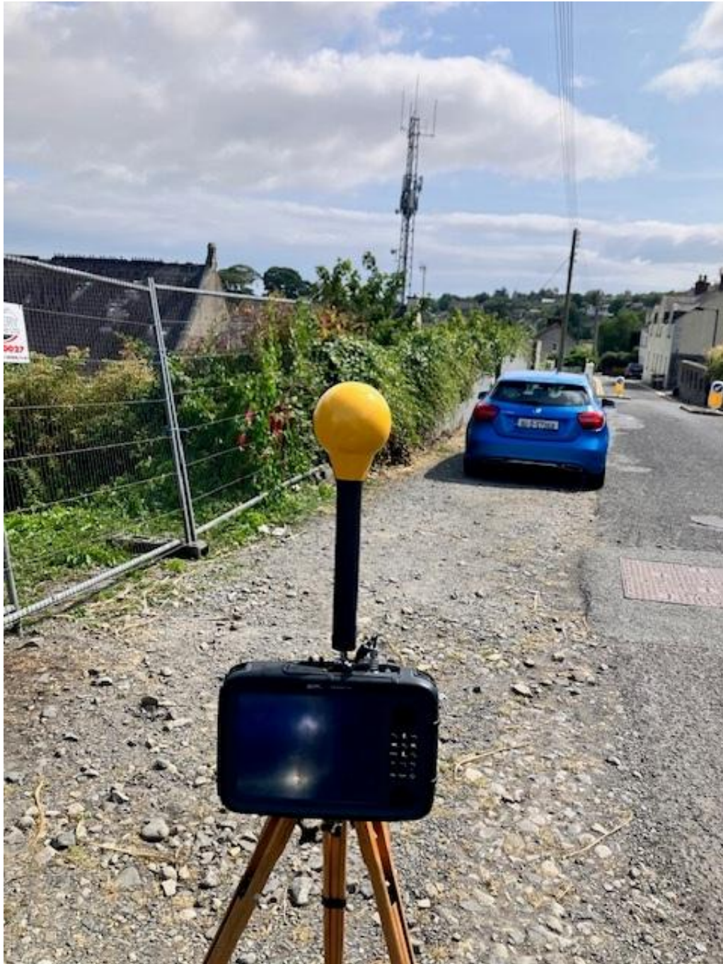
Photo 2. Frequency selective measurement location looking towards antennas
