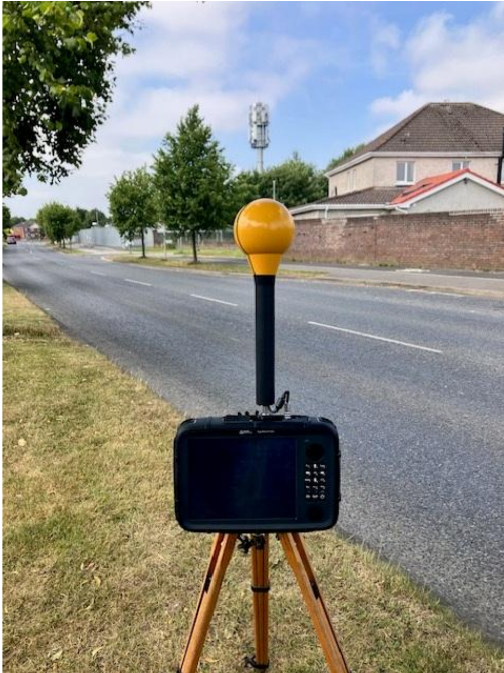
Photo 2. Frequency selective measurement location looking towards antennas
