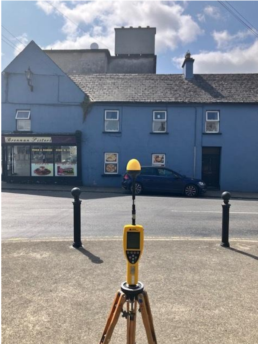
Photo 1. Broadband Measurement location looking towards antennas
