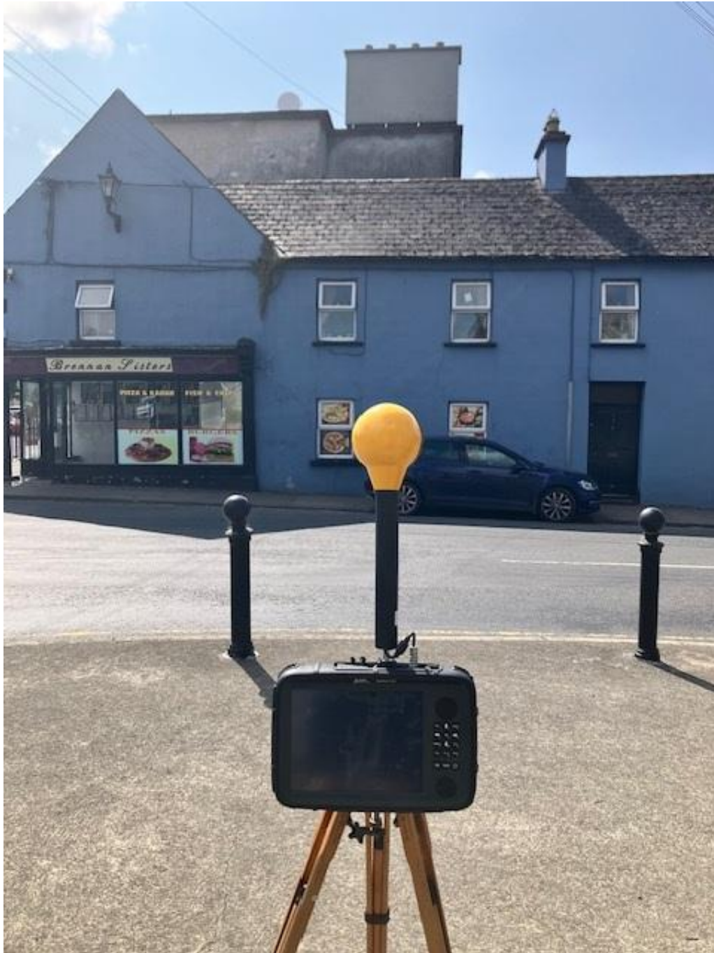
Photo 2. Frequency selective measurement location looking towards antennas
