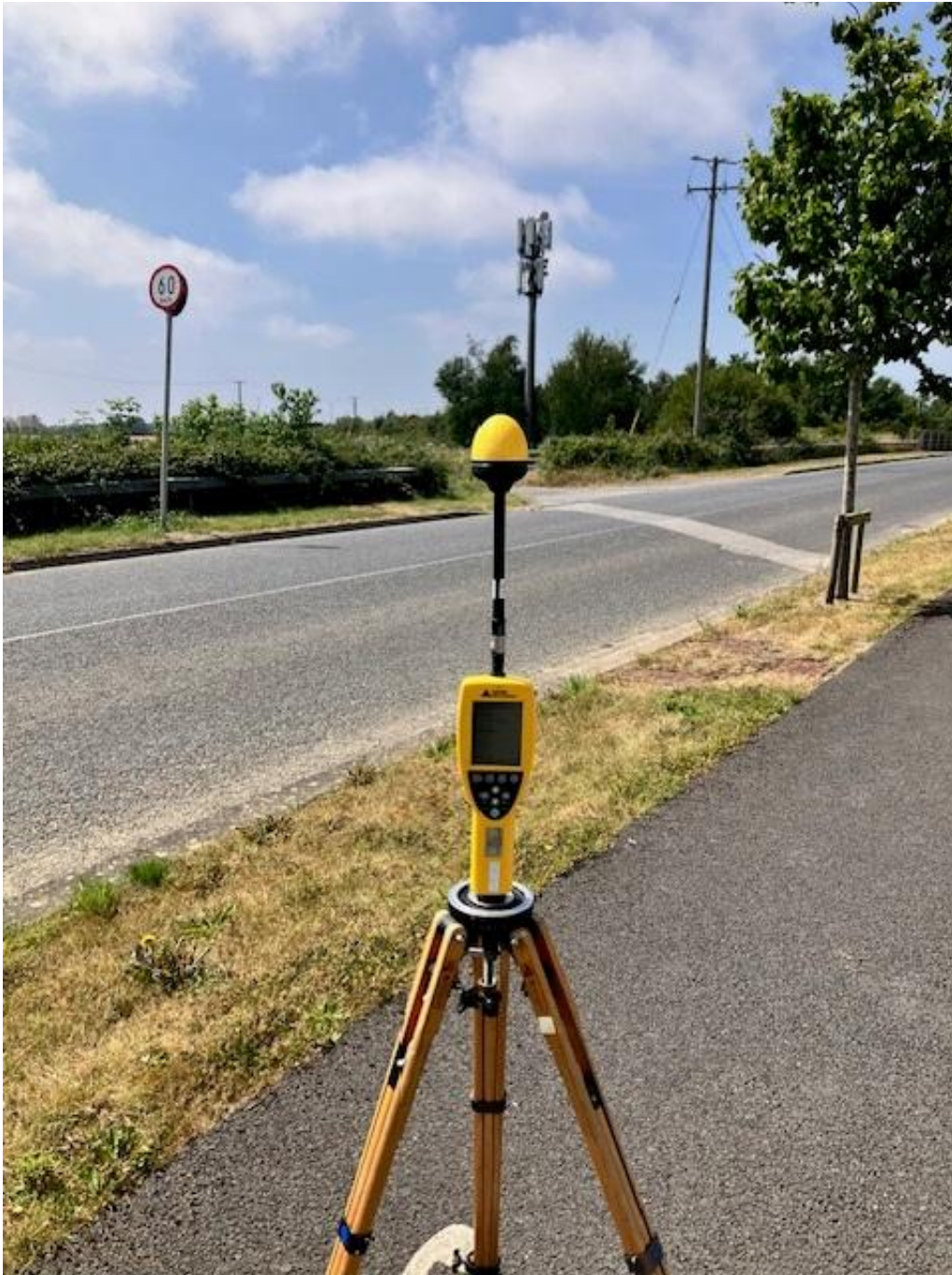
Photo 1. Broadband Measurement location looking towards antennas
