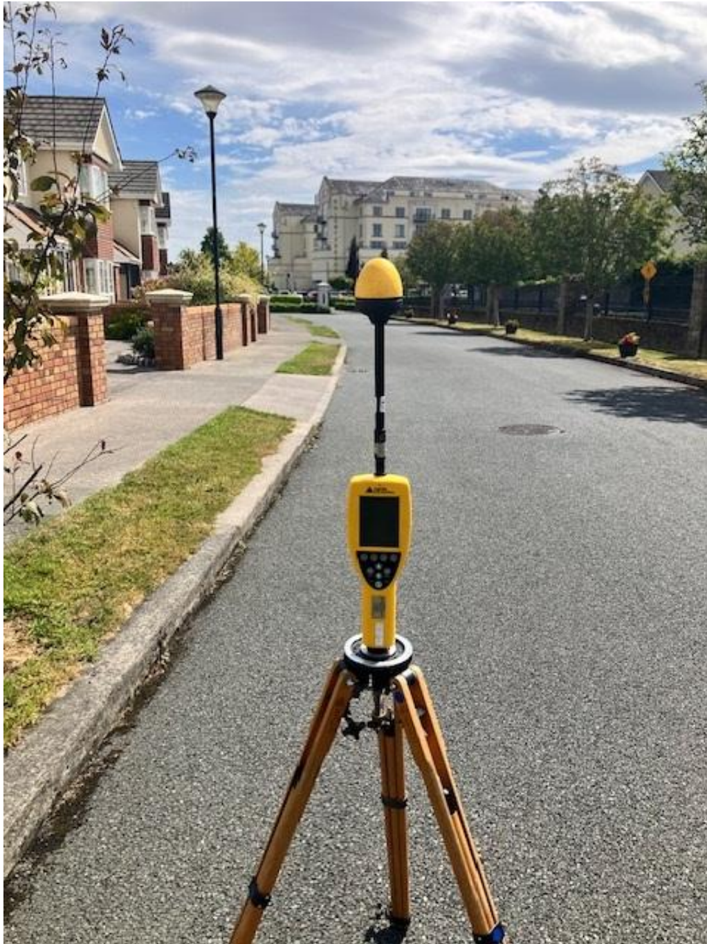
Photo 1. Broadband Measurement location looking towards antennas
