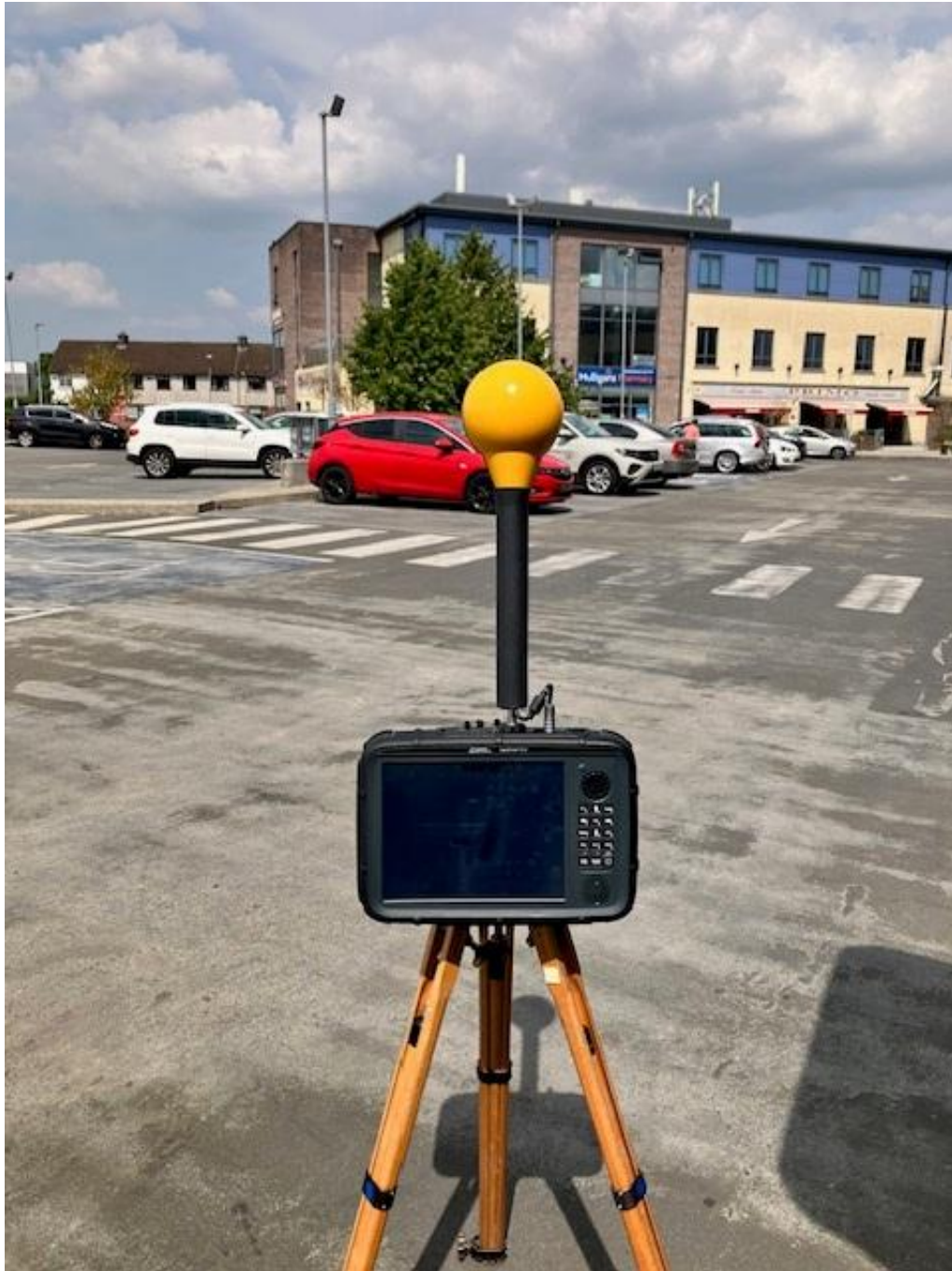
Photo 2. Frequency selective measurement location looking towards antennas
