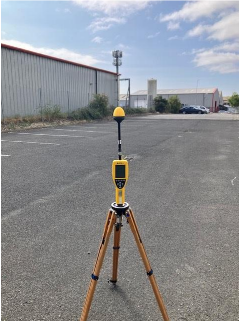
Photo 1. Broadband Measurement location looking towards antennas
