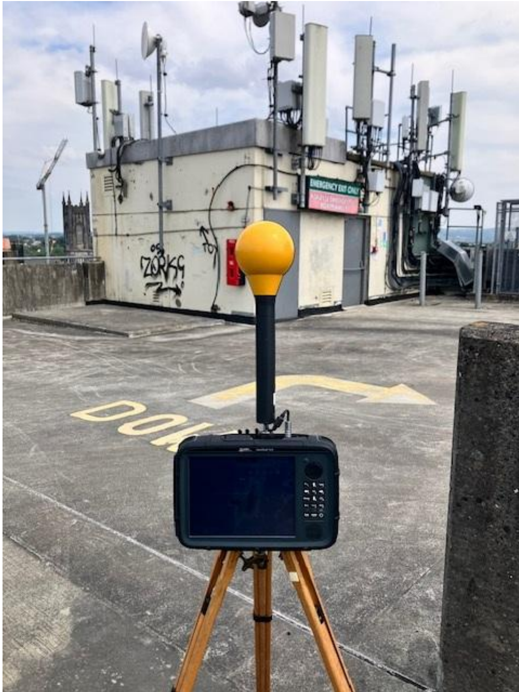
Photo 2. Frequency selective measurement location looking towards antennas
