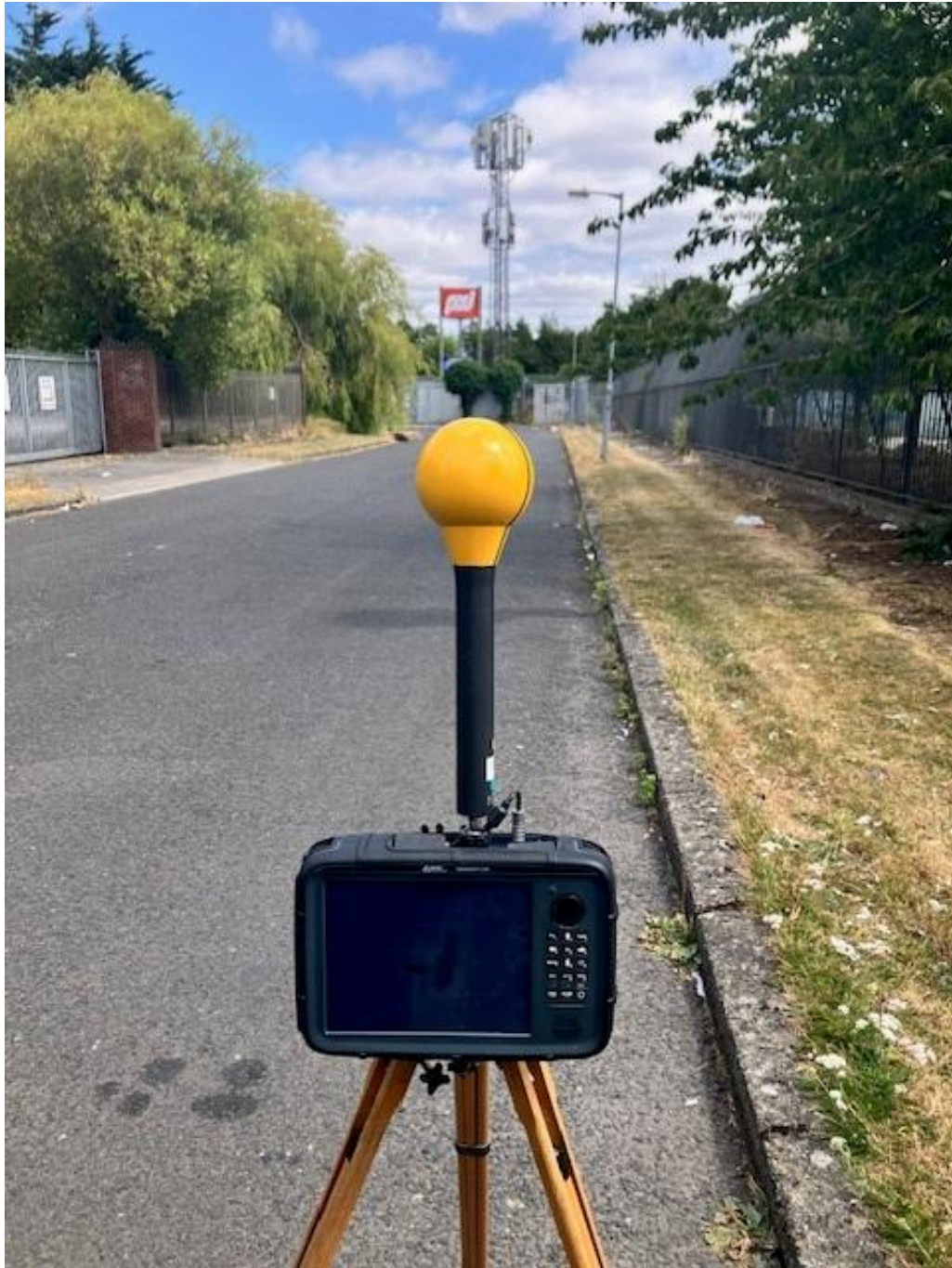
Photo 2. Frequency selective measurement location looking towards antennas
