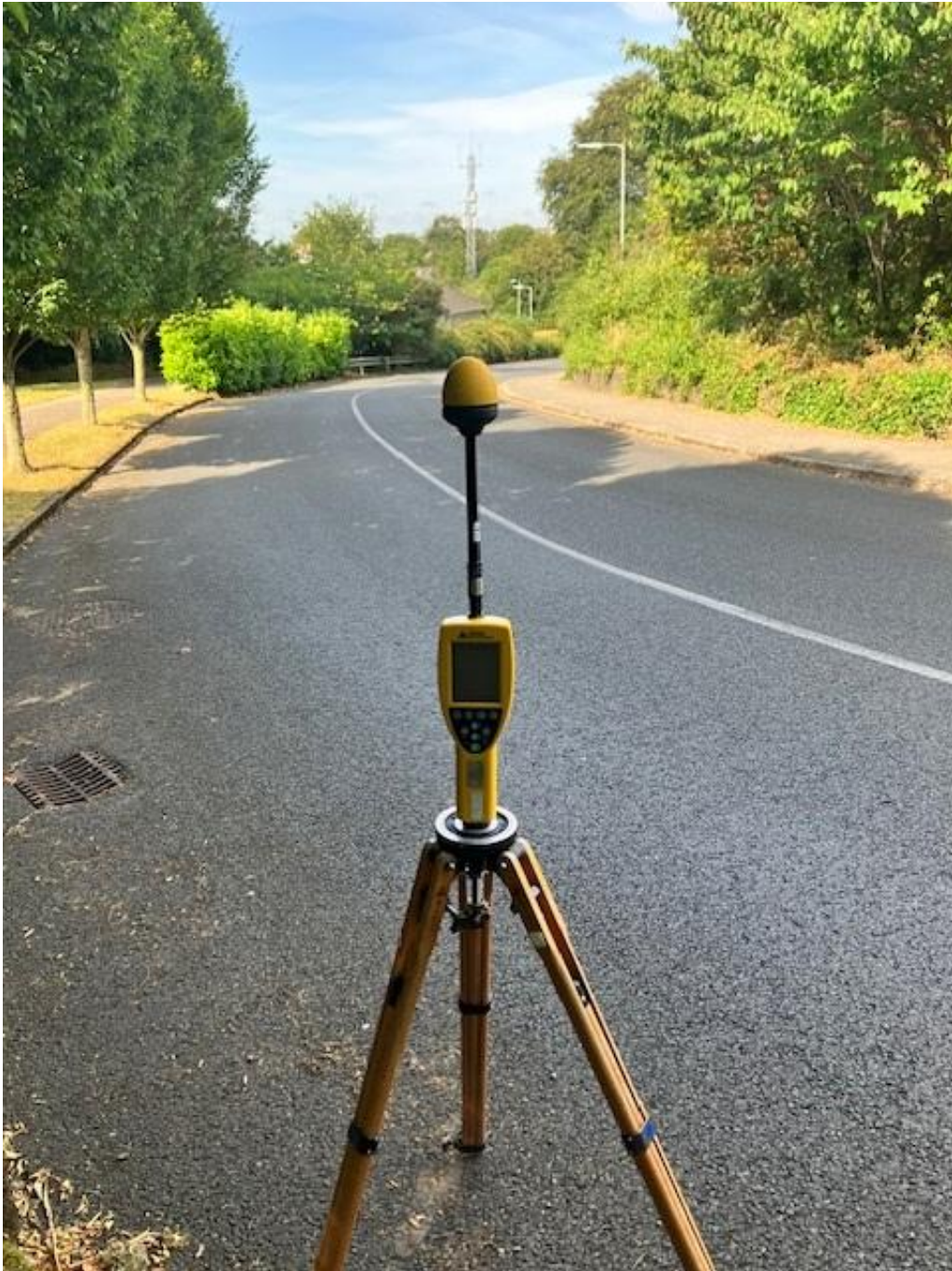
Photo 1. Broadband Measurement location looking towards antennas
