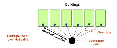
Figure 5 - Maximum distance between distribution points and buildings
