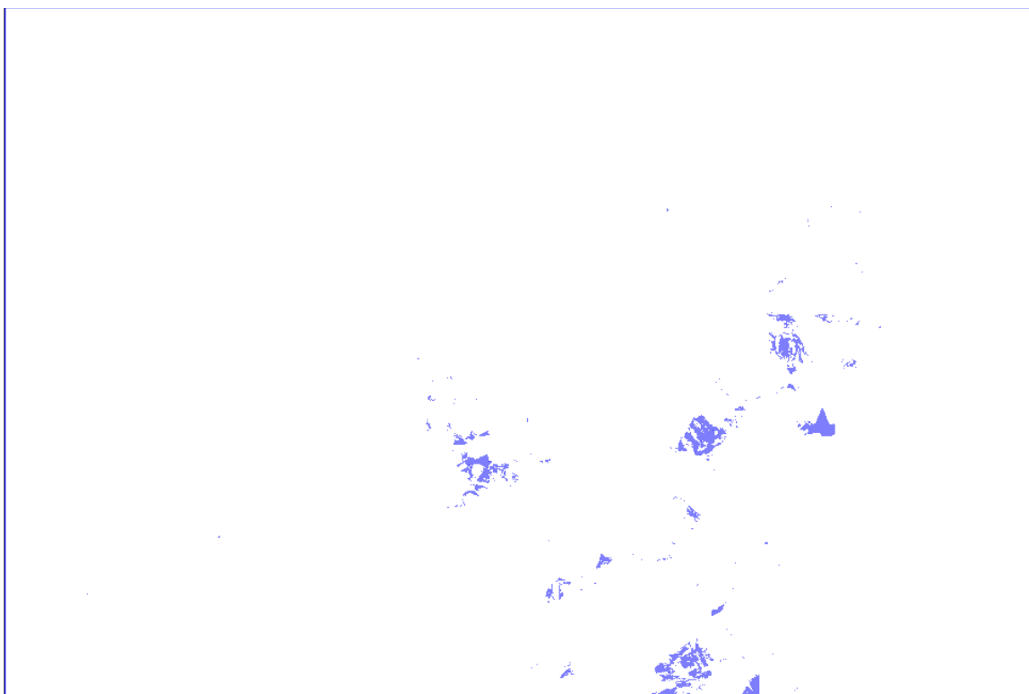
Figure 27: Rural Area C/Ic < 12 dB Interference Map; 50% GSM900 Traffic; 25 GSM channels; 12 TCH Channels C/Ic < 12 \text{ dB} = 77.76 \text{ km}^2
