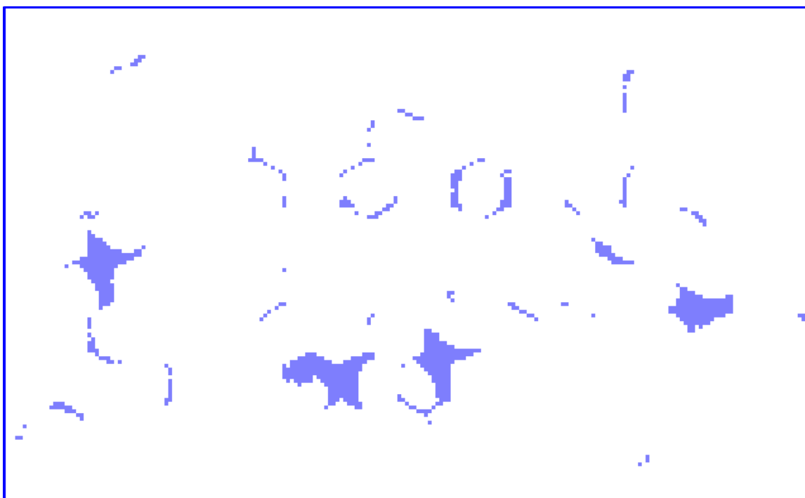
Figure 36: Urban Area C/Ic < 12 dB Interference Map; 60% GSM900 Traffic; 25 GSM channels; 13 BCCH Channels 45 Sites; C/Ic < 12 dB = 2.1 km 2
