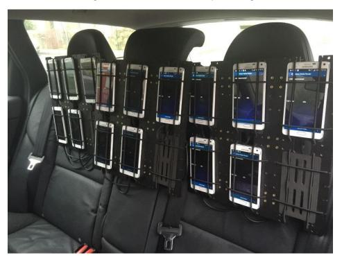
Figure 17: Measurement Set Up Showing Handsets
