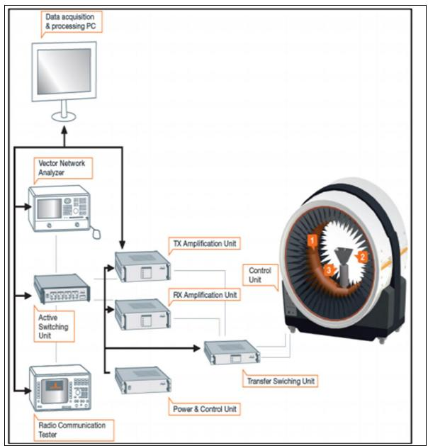
Figure 9: StarLab Test Setup<sup>45</sup>
