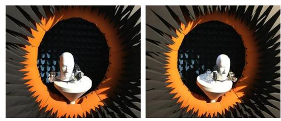
Figure 3: Handset Positioning for BHHL (left) and BHHR (right) scenarios
