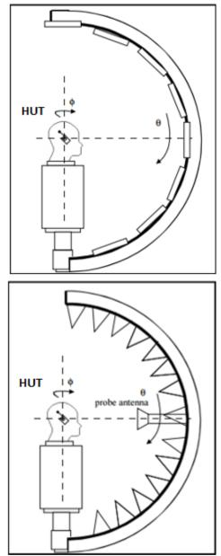
Figure 6: (a) Multi Probes (b) Single Probe (for illustration purpose)
