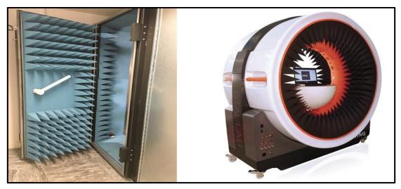
Figure 2: MVG StarLab Measurement System on the right was placed inside the Anechoic Chamber on the left for TRP and TIS Measurement<sup>29</sup>
