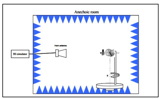
Figure 5: Dual axis system (for illustration purpose)
