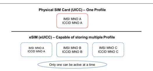
Note: There exist also physical SIM cards that can store multiple IMSIs, however, this is not the case with most SIM cards for the consumer market. Management of profiles, i.e. installation and deletion are not supported on the UICC. SIM profiles may also include security algorithms, OTA and authentication keys and other information used by the MNO. Source: GSMA (2018), eSIM Whitepaper – The what and how of Remote SIM Provisioning. WIK-Consult.
