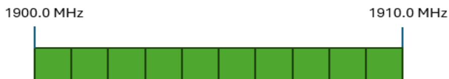
Figure 6: RMR 1 MHz TDD channel band plan in 1900 MHz
