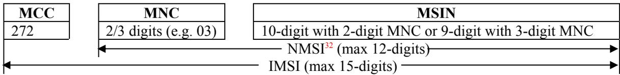
**Figure 5: The structure of the DNIC and terminal identifiers**
